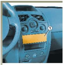
**Radio compartment 1** Unclip the blanking cover. The aerial, + and – supply and speaker wire connections are located behind it.
