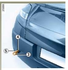
Access to towing rings Unclip cover 2 or 5.
