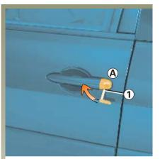
Using emergency key 2 built into the RENAULT card
