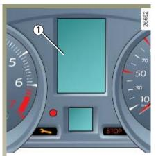
If the message "Check emission control" or "Regenerate particle filter" is displayed alongside the warning light, refer to your RENAULT dealer as soon as possible.
