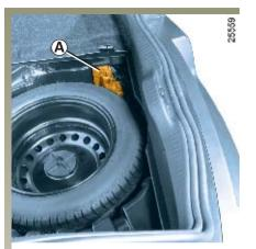
The tool kit *A* is located inside the luggage compartment to the right of the emergency spare wheel.
