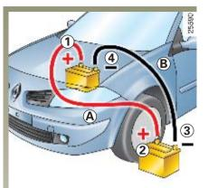
Secure the positive cable (+) *A* to the (+) **terminal** *1* of the discharged battery, then to the (+) **terminal** *2* of the battery supplying the current.
