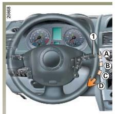
With the engine running or in the accessories position, move switch stalk 1.
