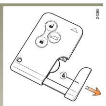
Integrated emergency key 4 or separate emergency key 5 (depending on the vehicle)
