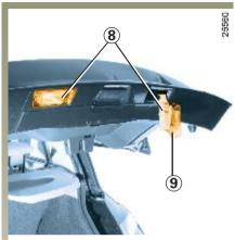
Number plate lights 8 Unclip light 8 by pressing tab 9. Remove the light cover to gain access to bulb.
