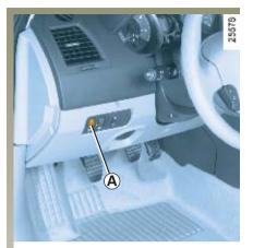
On vehicles equipped with this function, control knob A allows you to adjust the height of the headlight beams according to the vehicle load.
