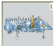
Front side light Remove bulb holder 7 to access the bulb.
