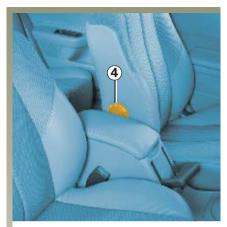
To adjust the lumbar support on the driver's seat Adjust control knob 4.
