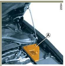
Certain functions are protected by fuses located inside the engine compartment (fusebox A).
