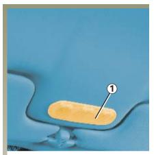
**Courtesy light** *A* Unclip transparent cover *1* (using a flat blade screwdriver type tool).
