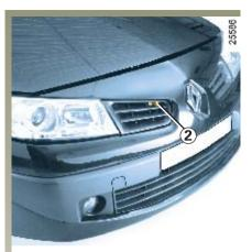
**Bonnet safety catch** To release, pull the tab that passes through the radiator grille panel **2**.
