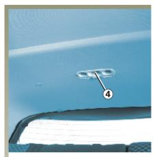
Remove the bulb concerned. Bulb type 4: W5W.
