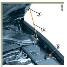
Lift the bonnet, release stay **4** from its holder **5** and, for your own safety, it is **very important** to fix it into retainer **3** in the bonnet.
