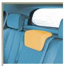
**Storage position** Press tab **1** and lower the head restraint completely.
