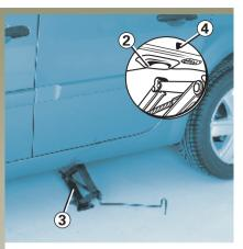
If necessary, remove the wheel trim. Undo the wheel bolts with wheelbrace **1**. Position it so that you can push it from above.
