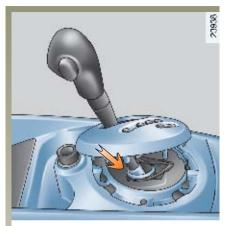
When setting off, if the lever is locked in position  $\mathbf{P}$  even though you are pressing the brake pedal, the lever can be released manually. To do this, unclip the upper section of the cover at the base of the lever.
