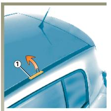
Each trim strip has two flaps. These flaps cover the mounting points for the roof rack bars.
