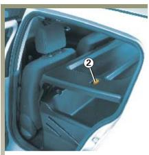
Special point for utility versions, unclip the fixings 2 from each side of the shelf, then take the shelf out through the rear door.
