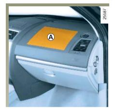
The airbag system uses the principles of pyrotechnics. This explains why, when the airbag inflates, it will generate heat, produce smoke (this does not mean that a fire is about to start) and make a noise upon detonation. In a situation where an airbag is required, it will inflate immediately and this may cause some minor, superficial grazing to the skin or other problems.
