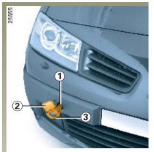
Only use the front 1 and rear 4 towing points (never use the drive shafts). These towing points may only be used for towing: never use them for lifting the vehicle directly or indirectly.
