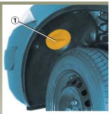
The bulbs can be accessed by removing blanking covers **1** and **2** located in the wheel arches.
