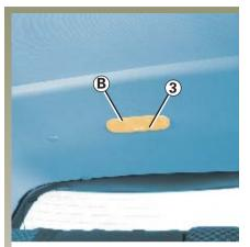
Courtesy light B Unclip transparent cover **3** (using a flat blade screwdriver type tool).
