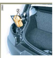
Release the rear light assembly from outside the vehicle by pulling it towards the rear.
