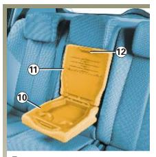
**Rear armrest storage** Lower armrest 10 and lift cover 11 using release handle 12.
