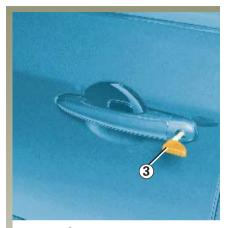
Using the separate emergency key 3 (depending on vehicle) Insert key 3 into the lock of the lefthand door and lock or unlock the door.
