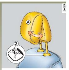
To remove the head restraint
