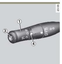
Switching on the dipped beam headlights
