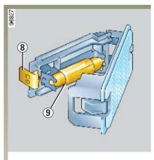
Press tab **8** to release the bulb holder and gain access to the bulb **9**.
