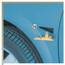
**Side-mounted indicators 10** Unclip indicator **10** (using a flatbladed screwdriver or similar tool). Turn the bulb holder one quarterturn and take out the bulb.
