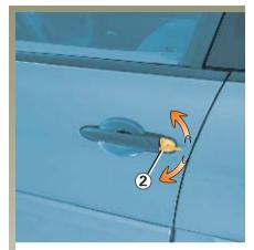
Insert key **2** into the lock of the front left-hand door and lock or unlock.
